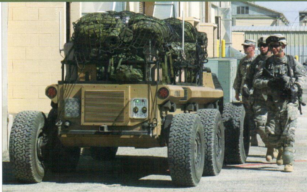
Soldiers of the Army Evaluation Task Force at Fort Bliss test the Multifunctional Utility/Logistics and Equipment (MULE) vehicle. The MULE is a three-ton unmanned ground system designed to support dismounted, mounted and air assault operations. (Army photo)
